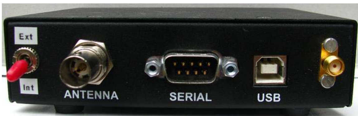
Fig 5 – View of SDR-IQ rear panel, showing LO switch and input connector
