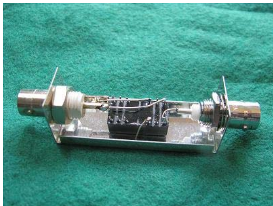
Fig 5 – A recovered filter assembled in a small tin-plate enclosure, with insulated output connector
